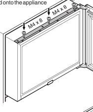
4. Slide the appliance into the recess leaving a 21 mm gap between the body of the unit and the front face of the door.
